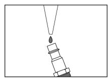
Figure 9. Lubricating nailer/stapler via air inlet.
